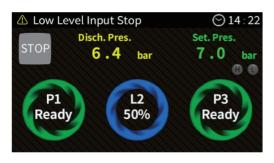
In order to detect the low water level in the suction pipeline, change the INPUT 6 to suction IvI H and INPUT 7 to suction IvI L. To measure the discharge water level, change the INPUT 6 to discharge IvI H and INPUT 7 to discharge IvI L.
