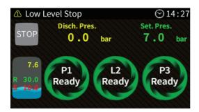
Change the sensor 3 to level sensor to utilize the water level sensor. Once this is set, a level icon should appear on the main operation screen.
