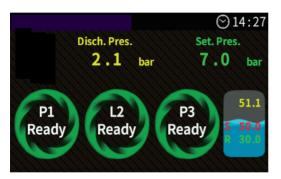
\* Note: If the value of the stop level is greater than the value of the operation level, the system will operate on discharge level and vice versa. With this said, the level icon will change from left to right depending on the setting.
